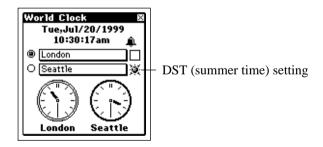
On the clock screen, tap on the DST (summer time) setting of one of the clocks to toggle it between DST on ( $\bigotimes$ ) and DST off (no indicator).
