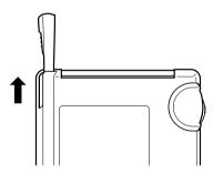
7. Open the cover and touch the screen with the stylus to turn on power.
