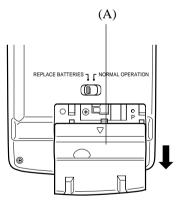
3. Load two new batteries, making sure that their positive (+) and negative (-) ends are facing in the proper directions.
