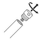
2. Insert the battery with the positive (+) terminal towards the tip of the pen.
