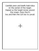
Press the stylus against the center of the target mark (+ mark) as indicated on the screen. The screen shown below appears after you press the stylus against the target at five different locations.
