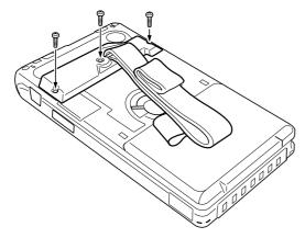
Attach the strap using the strap hole in the bottom of the IT-600.
