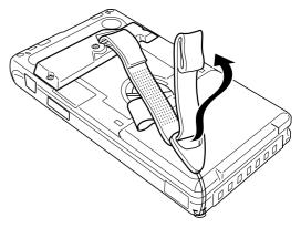
5 You can also use the strap to hold the stylus when required, as shown in the figure.
