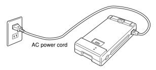
2. Mount the battery pack onto the AC adapter/charger.
