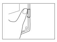
If the raised part of the jack cover is not completely inside of the groove, press it into place by running your fingertip along the cover.
