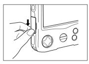
While continually applying pressure, slide your finger to the other side of the cover so it closes completely.
