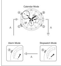
Use (A) to navigate between modes. Hold down (A) for about two seconds to enter the Calendar Mode. To connect with a phone, hold down (C) for about 0.5 seconds.
