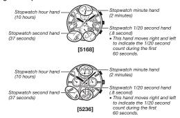
The stopwatch lets you measure elapsed time up to 11 hours, 59 minutes 59.95 seconds.
