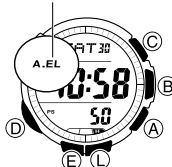
Auto light switch on indicator
