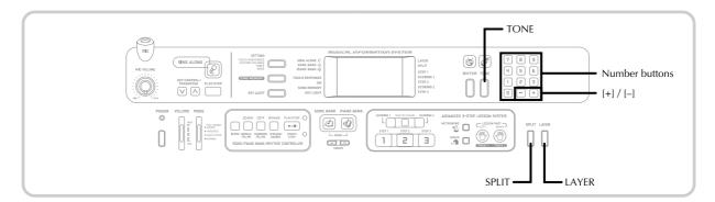
This section describes how to use layer (to play two tones with a single key) and split (to assign different tones to either end of the keyboard), and how to make touch response, transpose, and tuning settings.
