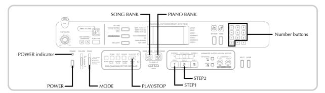
This section provides a quick overview of keyboard operation using steps one and two of the 3-step lesson feature.
