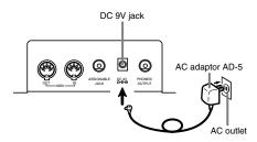
Also note the following important warnings and precautions when using the AC adaptor.
