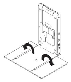
$\ensuremath{\textbf{3.}}$  Unfold the camera holder from the arm unit.
