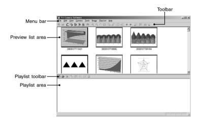
The following explains the main functions of PJ Camera Software window components.
