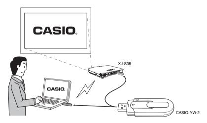
You can have up to four computers connected to the Data Projector over a wireless LAN at the same time. Use the remote controller that comes with the Data Projector to select which of the four computer screens you want to project.
