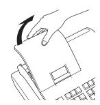
**2** Remove the battery compartment cover.
