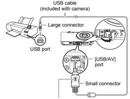
Making sure that the 1 mark on the USB cable connector is towards the lens side, connect the cable to the camera.
