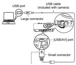
Making sure that the 1 mark on the USB cable connector is towards the lens side, connect the cable to the camera.
