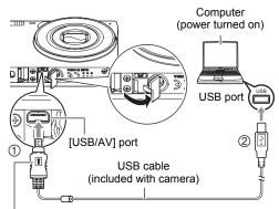
Making sure that the 1 mark on the USB cable connector is towards the lens side, connect the cable to the camera.
