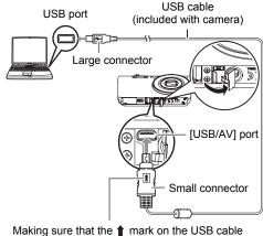
Making sure that the 1 mark on the USB cable connector is towards the lens side, connect the cable to the camera.
