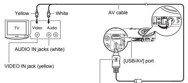
Making sure that the  $\Uparrow$  mark on the AV cable connector is towards the lens side, connect the cable to the camera.
