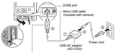
• mark of the small (micro USB) connector facing the monitor screen side of the camera.
