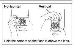
This is especially important when available lighting is low, which slows down the shutter speed.
