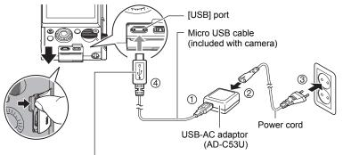
• mark of the small (micro USB) connector facing the monitor screen side of the camera.
