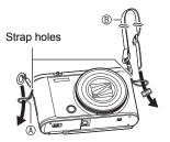
**3.** Pass the end of the strap through the strap loop ring (A) and secure it with the buckle.
