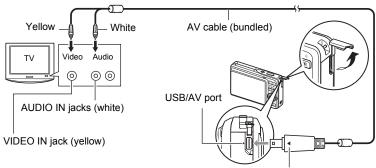
Making sure that the ▶ mark on the camera is aligned with the ◀ mark of the AV cable connector, connect the cable to the camera.
