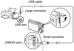
Making sure that the ▶ mark on the camera is aligned with the ◀ mark of the USB cable connector, connect the cable to the camera.
