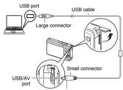
Making sure that the ▶ mark on the camera is aligned with the ◀ mark of the USB cable connector, connect the cable to the camera.
