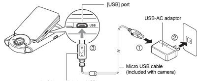
• mark of the small (micro USB) connector facing the side opposite that of the monitor screen.
